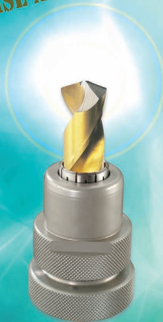
NACHI SG-ES Drill Point Style: 3 rake angles and split point
