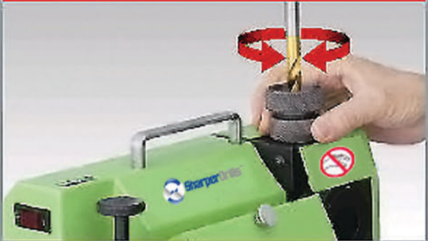
Second: Grinding The Relief (Web Thinning)
