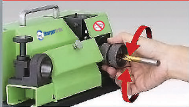
First: Grinding The Drill Point In One Step
