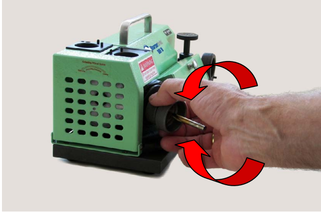
Third Operation: Grinding Split Point (X-thinning)
