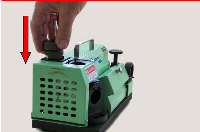
Third Operation: Grinding Split Point (X-thinning)
