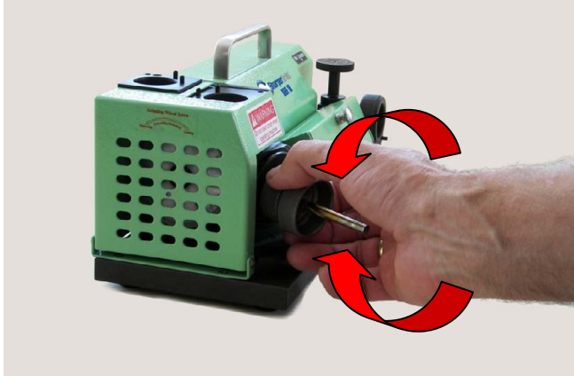
Third Operation: Grinding Split Point (X-thinning)
