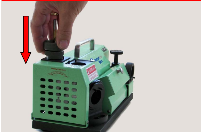
Third Operation: Grinding Split Point (X-thinning)
